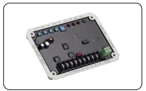
Digital Governor for use in Gas and Diesel Generators with smoke and IDLE controls. Senses generator frequency, no magnetic pickup unit (MPU) is required. Applicable to all types of generator engines and also supports External, Internal, and PT Pump mounted actuators.
